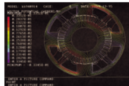
Magnetic Flux Vector Potential in core
